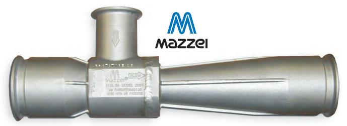
Made from cast stainless steel, the model SS-2081 has 2" triclamp wine-line connections, and a 1 1/2" suction connection. Wine pumped through the injector creates a vacuum after the throat of the device, in turn creating suction through the lateral port.
